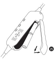
This product is built for use with regular disposable batteries. Reachable batteries or lithium batteries may be used but may influence the correct function of the low power indication. Please note that rechargeable batteries cannot be charged in the PM6 control module.
